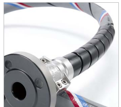
KSS Anti-Kinking Spiral with suitable Spannlloc KSS clamps. Patented system for tightly bent hoses - protects the stressed area directly behind the coupling (see Elaflex Information 2.09 E)
